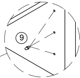
Note: the iron can put three adjustable positions for middle shelf level.
